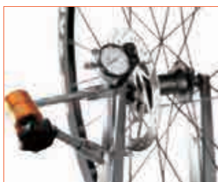
To measure and true disc brake. *NOTE: Turn the knob to loosen the arm before using everytime
