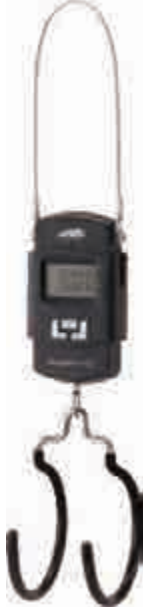
TB-DS10 Digital scale •The versatile digital scale is designed to measure accurate weight of bikes, frames and components. •Perfect to work with Super B work stands. •Measures weight range from 20g ~ 50 kg with kg / lbs. unit conversion. •Accurate to ± 5 g from 20 g to 10 kg, ± 10 g from 10 kg to 50 kg. •Tare and auto power-off function. •Requires 2 AAA batteries that are not included.
