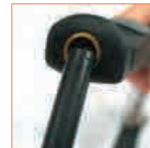
Housing Reformer for easy installation of ferrules.
