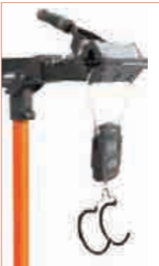
TB-DS10 Digital scale •The versatile digital scale is designed to measure accurate weight of bikes, frames and components. •Perfect to work with Super B work stands. •Measures weight range from 20g ~ 50 kg with kg / lbs. unit conversion. •Accurate to ± 5 g from 20 g to 10 kg, ± 10 g from 10 kg to 50 kg. •Tare and auto power-off function. •Requires 2 AAA batteries that are not included.
