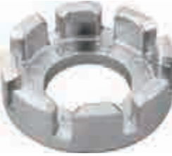
TB-5502 Aero spoke key •Deep slots fit wider Aero spokes. •Steel core covered with nylon prevents the flat spokes turned when adjusting the nipple of spoke. •A ring design makes easier and more stable operation when wearing on the finger. •Aero spoke key 0.9 / 1.1 / 1.3 / 1.8 mm.
