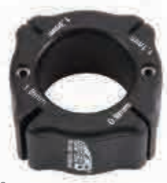
TB-5501 Aero spoke key •Steel core covered with nylon prevents the flat spokes turned when adjusting the nipple of spoke. •A ring design makes easier and more stable operation when wearing on the finger. •Fix Aero spoke, size: 0.9 / 1.1 / 1.3 / 1.9 mm.
